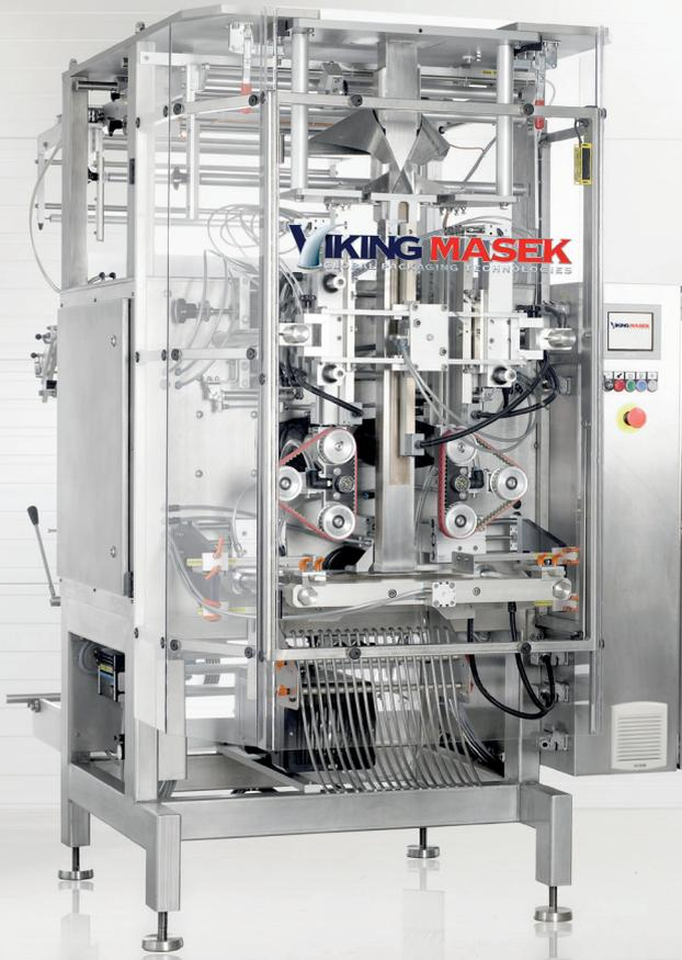
The M400, one of our most versatile baggers, is able to make quad seal, flat bottom, doy style, brick fold down / tape down, and pillow bags – all on one machine. The M400 is a robust stainless steel machine capable of running large bags up to 400 mm wide and 500 mm long.
