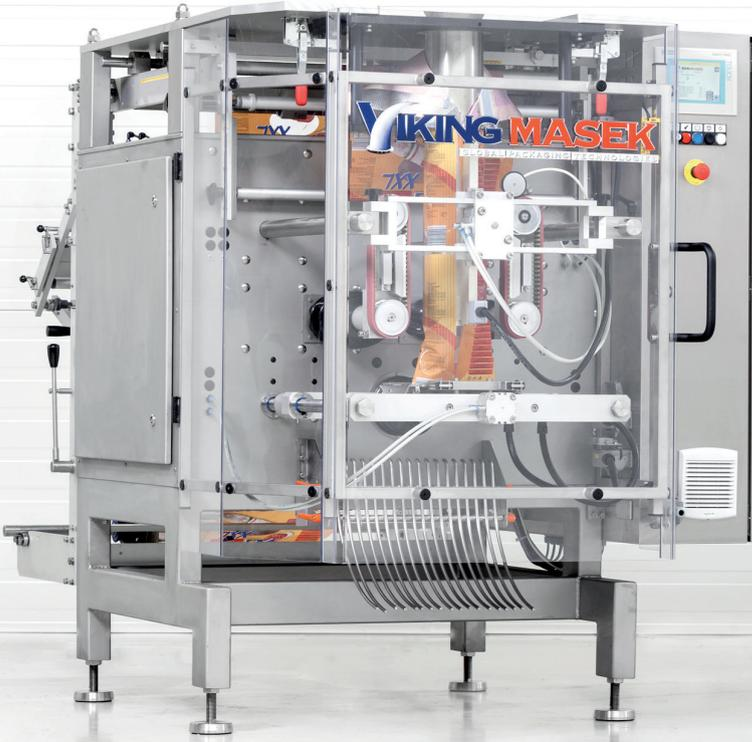
We used our broad engineering expertise to design our M-series VFFS machines. The M250's rugged construction and enclosed jaw drive makes this VFFS bag-maker an excellent choice for dusty or wet environments.
