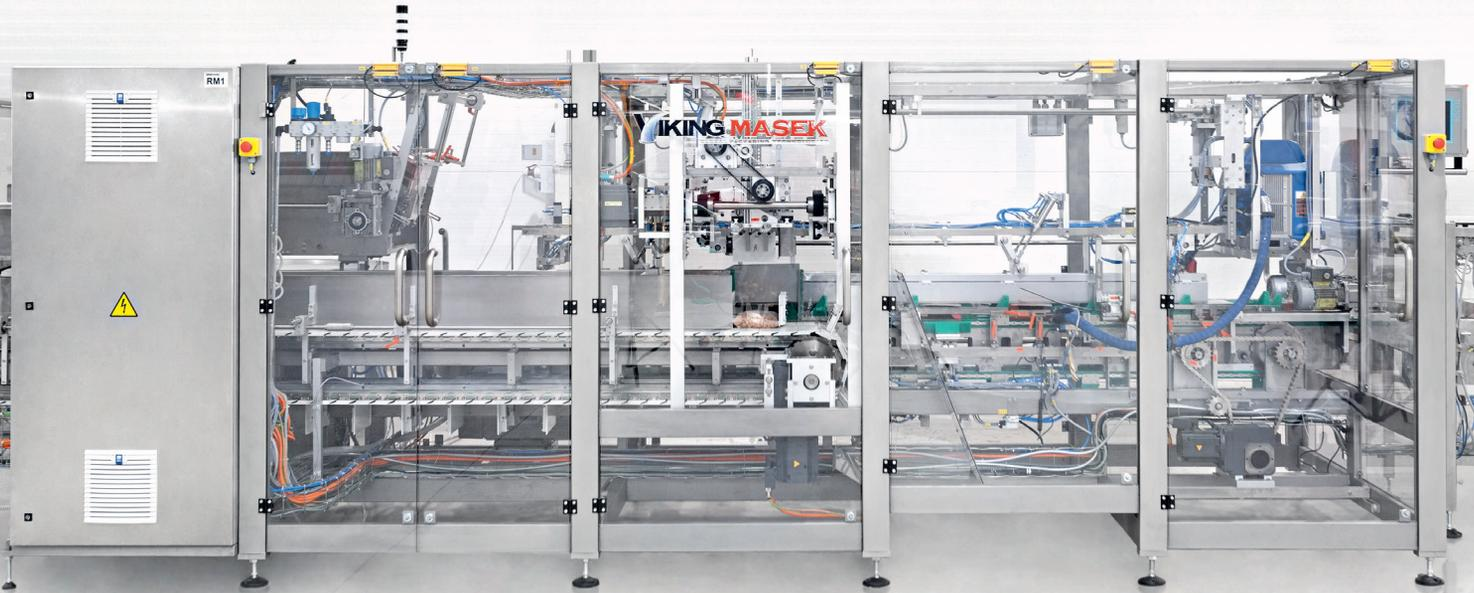
Viking Masek's CAM cartoners are fully servo driven, automatic continuous or intermittent endload cartoners, carefully designed to match specific applications on exact speed and size range requirements.
