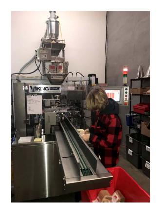
pouch machine was able to open and reclose the zipper seal and fill Bean Box's 2-ounce bags without either wrinkling or tearing the paper pouches.
